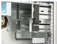
Quick-Release Drive Cage Tool-Less Design
