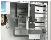
Quick-Release Drive Cage Tool-Less Design
